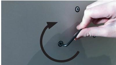
Fasten the screws by turning clockwise. Beware not to overtighten.
