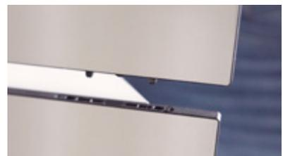
Align the pins of the top module with the notch in the bottom module.
