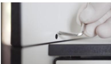
Use the Allen key to fasten the joints in all four corners...
